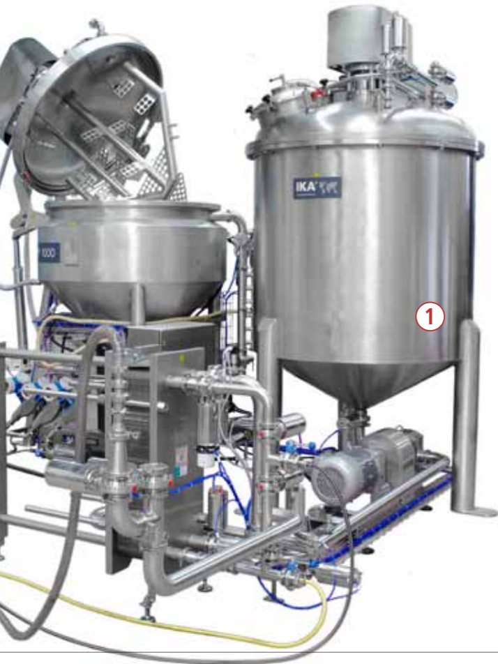
① Buffer tanks available with or without agitator, double jacket and temperature control function for storage of your intermediate or final product
